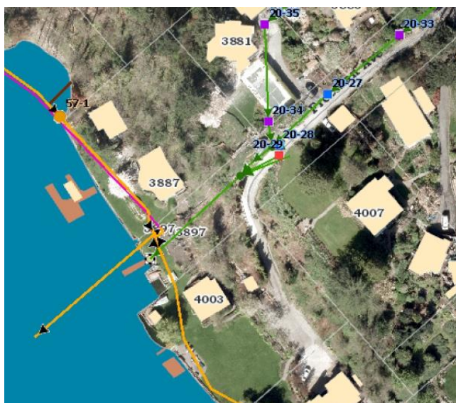
Figure 3: Screen shot of the City of Mercer Island Public Works IGS Utilities Map showing existing stormwater and sanitary sewer utilities.
